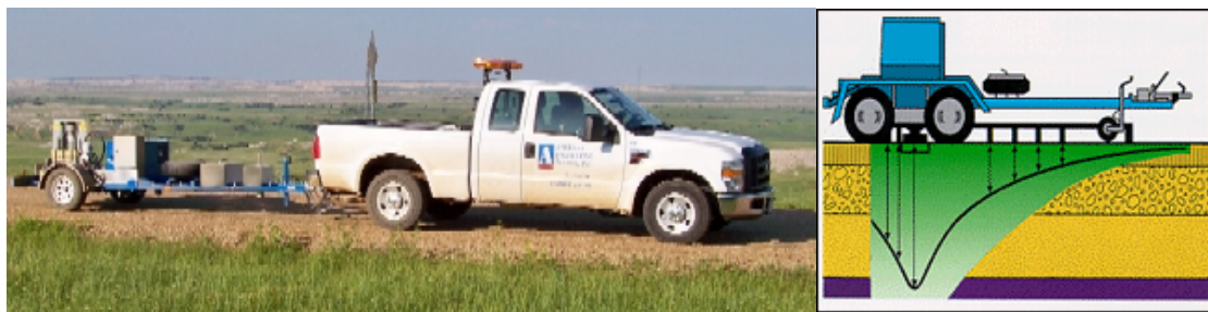
Figure B1 Dynatest 8002 FWD Test System
