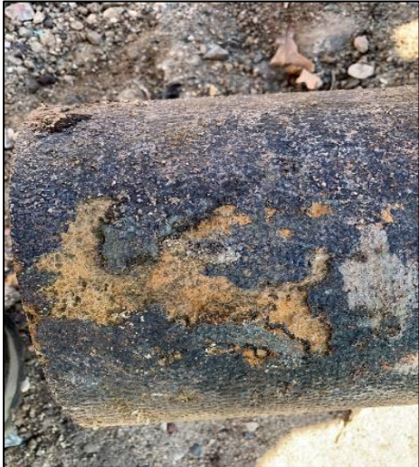
Ductile iron watermain in project area corroded down to concrete pipe liner
