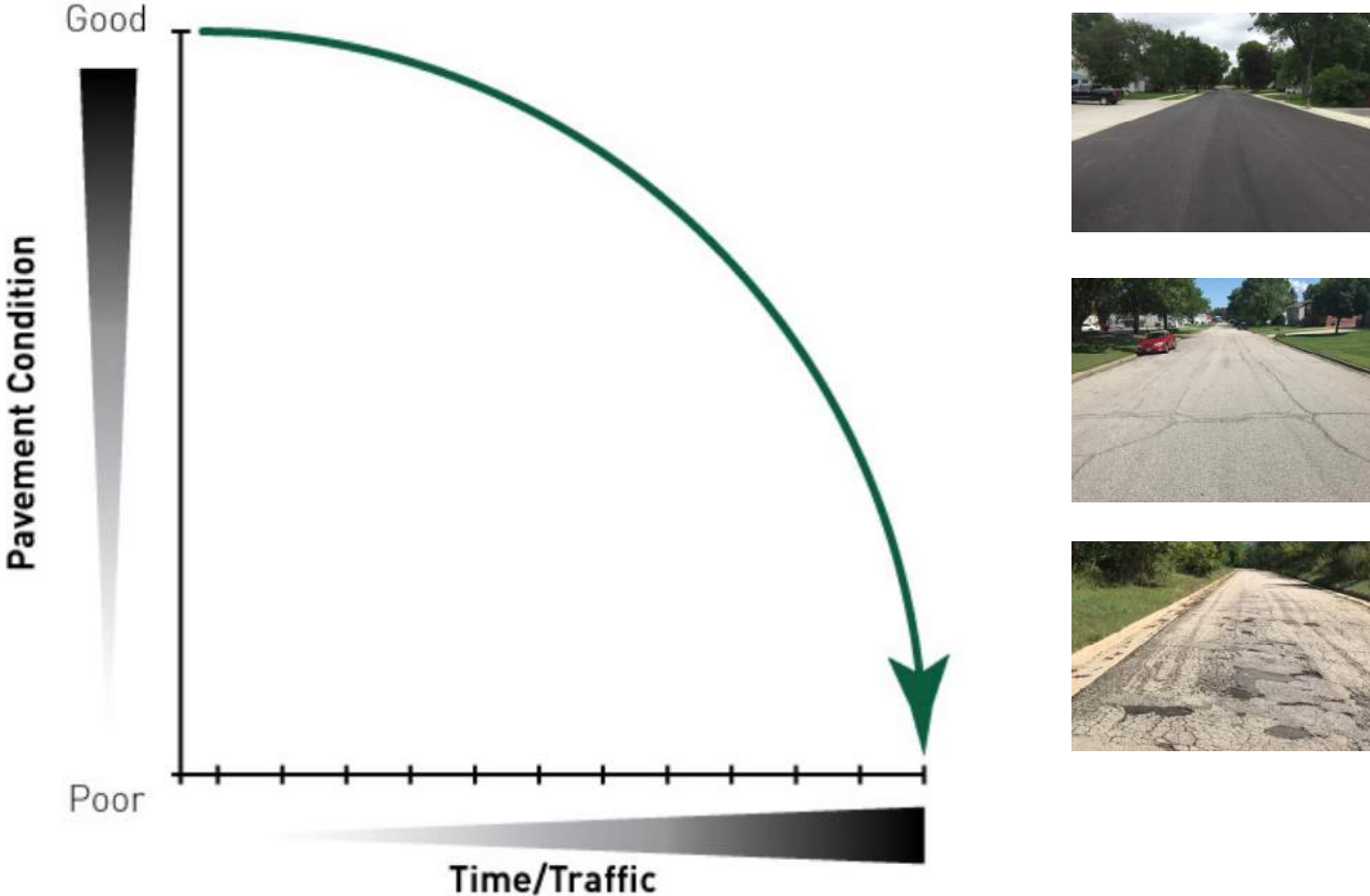
Figure 1: Typical Pavement Lifecycle No Seal Coat, Crack Fill or Overlay
