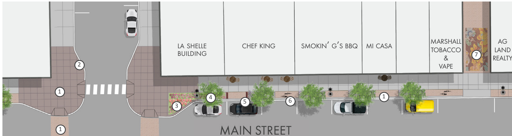
Illustrated plan view of Main Street between 1st Street and Center Street. Removing the large sidewalk canopy attached to the Le Shelle and Chef King buildings provides space for street trees and outdoor dining while also featuring improved business visibility.
