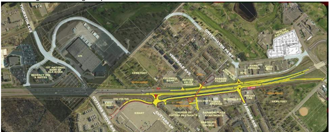
Figure 1. Stage I: Fairoak Ave traffic signal removal, construction of a reduced conflict intersection at Fairoak Avenue, a frontage road from Cutters Grove to Fairoak Ave, and a pedestrian overpass near Verndale Avenue. Source: Highway 10 Access Planning Study, Fairoak Traffic Signal Removal, p. 81)
