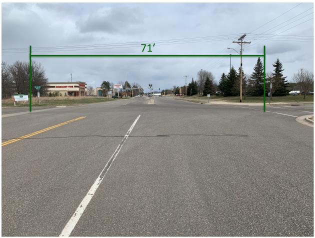
Figure 2: Glory Road Lane Configuration with Intersection width
