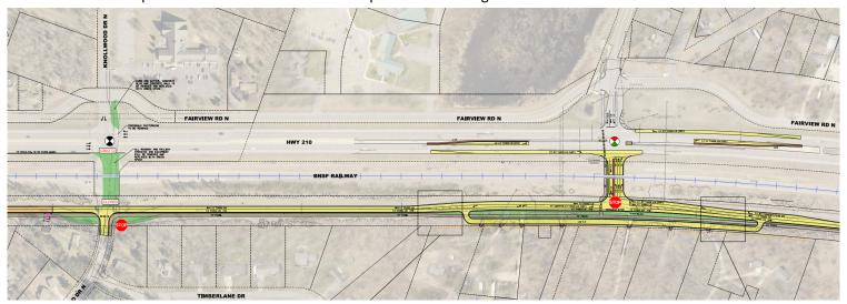
Figure 1: Plan View of Proposed Project. Closure of the South Leg on Knollwood Drive with a replacement at Inglewood Drive
