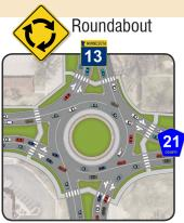
The intersection control alternatives at TH 13 and CH 21 include an improved signalized intersection (additional turn lanes and signal retiming) or a multi-lane roundabout.
