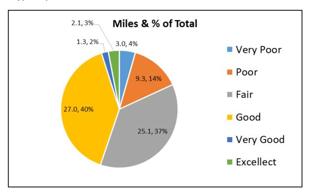
The Committee worked with Bolton & Menk to look at modifying the 2008 Pavement Management Plan to address the roads that are in the greatest need. The plan calls for the reclaiming and repaving all of the roads rated very poor or poor with ditch-to-ditch improvements in 2018 and then providing for a mill and overlay of the road surfaces that are currently rated fair in 2020, 2021, and 2022.
