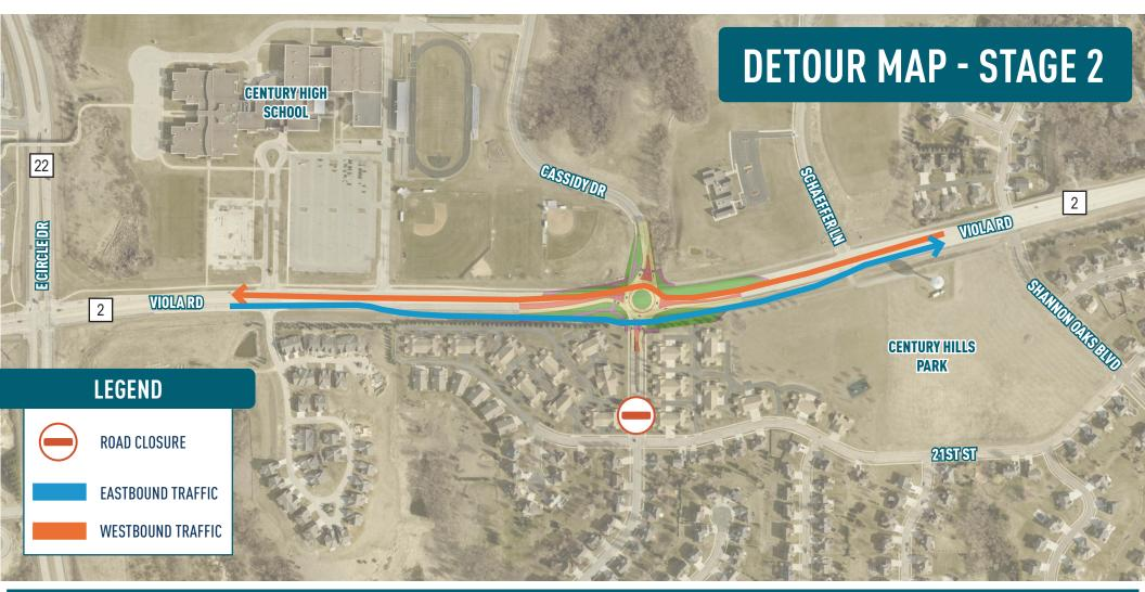
During Stage 2, all side streets on the north side of Viola Road are now open. Westbound traffic is driving through the roundabout on new pavement. Eastbound traffic remains on the eastbound shoulder and temporary paving while the south half of Viola Road and the roundabout are constructed.
