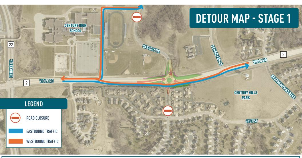
Stage 1 allows local access to Cassidy Drive utilizing Century High School's interior roadways. Temporary traffic control and pedestrian crossing enhancements will be implemented. The north half of Viola Road and Cassidy Drive are constructed at this time. Through traffic on Viola Road is shifted to the eastbound shoulder and temporary paving south of the roadway.
