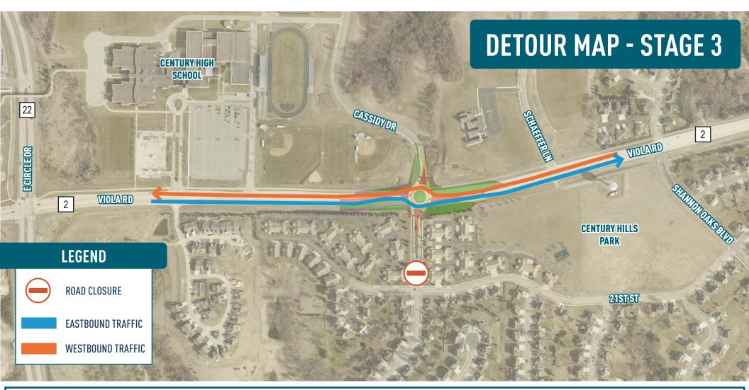
During Stage 3, all side streets on the north side of Viola Road are now open. Eastbound and westbound traffic is driving in the roundabout on new pavement. The south leg of the roundabout on Century Hills Drive is constructed, temporary pavement is removed, and the trail on the south side of Viola Road near the intersection is constructed.
