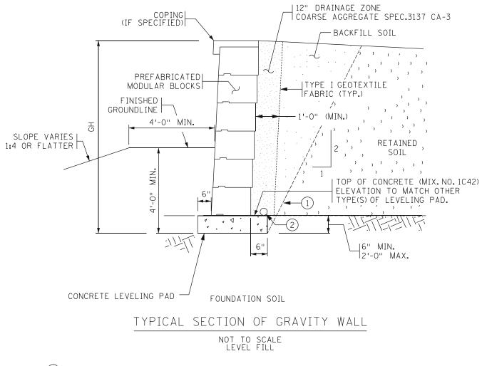
(1) PAY LIMIT (2:V TO 1:H) ACTUAL EXCAVATION SLOPE IS DETERMINED BY DESIGNER PREFERENCE OR OSHA REGULATIONS OF IN-SITU SOILS: EXCAVATION BEYOND THESE LIMITS AT CONTRACTORS EXPENSE.
